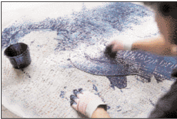
Resin infilling into names sandblasted onto a terrazzo disc
