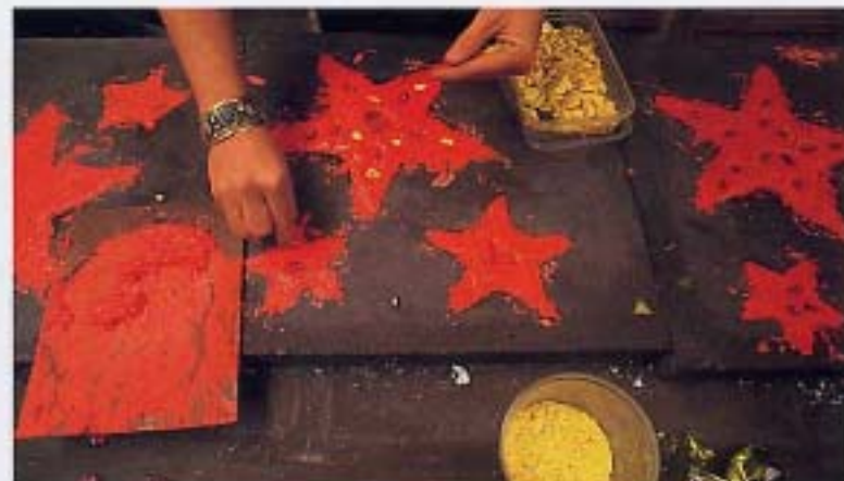
Insetting coloured glass chips into concrete star tiles
